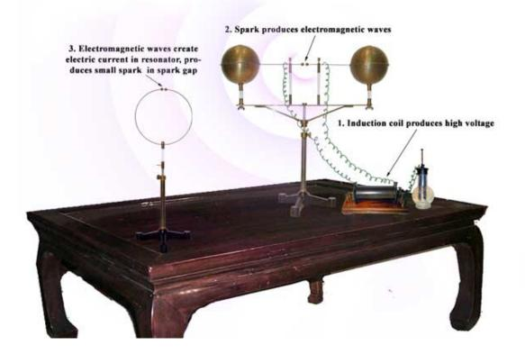
The ring at the left detects the waves. The ring is not completely closed: there is a small gap. The waves cause small sparks to be seen jumping the gap. If the ring is turned ninety degrees, you don't see the sparks, showing that the waves are "transverse waves",
